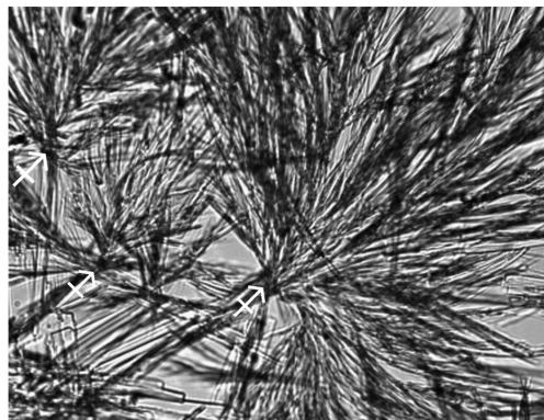
Fig. 4 Cholesterol anhydrous, recrystallized from dry methanol. At the end of needle-like crystals (crossed arrows) new needle-like crystals grow to form arborescent structures
